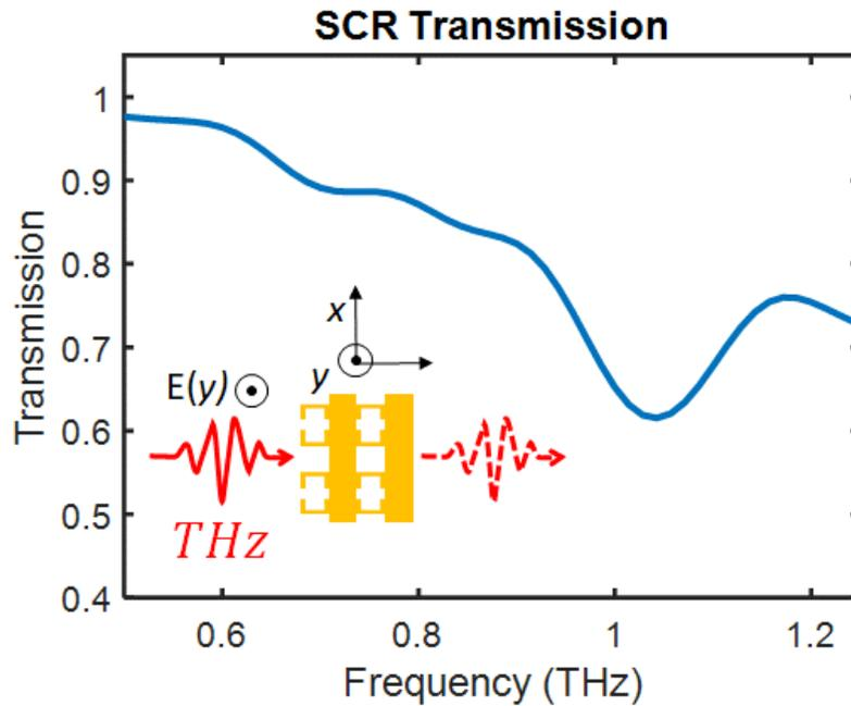
**Fig. 3.** Experimental transmission measurements of 3D THz MM. Normalized transmission of the free-standing SCR MM structure, see inset (twelve layers of SCRs are present in the sample, for simplicity we show only four). The IP-S polymer scaffold is conformally coated with 500 nm of ZnO via ALD.
