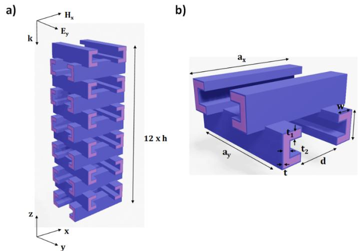
**Fig. 4.** Structure of split-cube-resonator (SCR) metamaterial. (a) Structure used for simulations, composed of twelve layers of SCRs. (b) Unit-cell of the periodic structure with annotated geometrical parameters.
