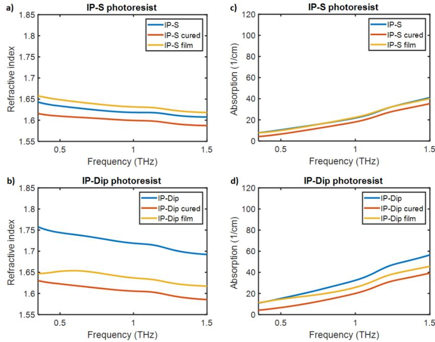
**Fig. 2.** Measured dispersive refractive index  $n(\omega)$  and absorption  $a(\omega)$  of IP-S and IP-Dip at the THz range. a-b)  $n(\omega)$  and c-d)  $a(\omega)$  measurements of IP-S and IP-Dip photoresists. In all cases, blue, red, and yellow stand for uncured, cured, and resists measured as cured thin films.
