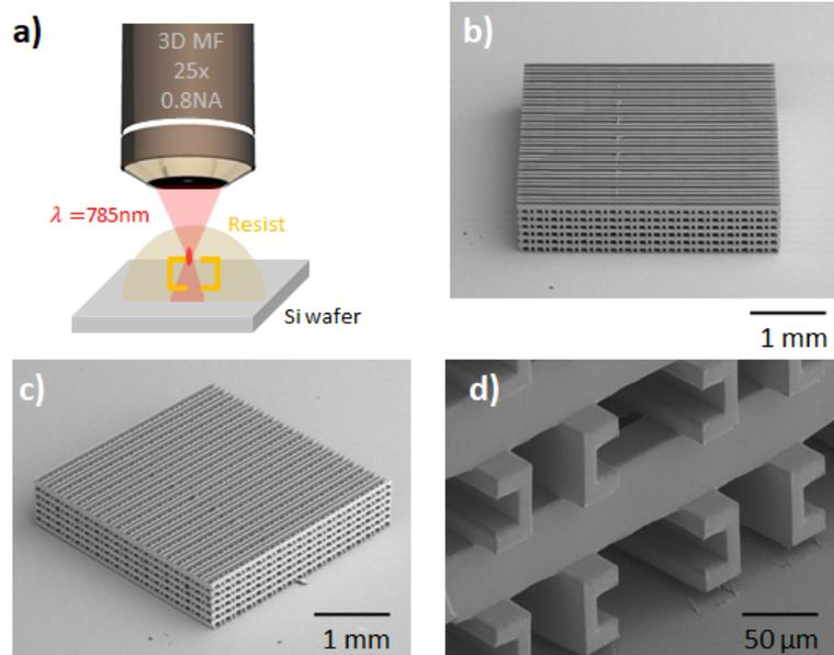
**Fig. 1.** Laser-processed THz mm-scale metamaterials (MMs). a) Direct laser writing (DLW) of 3D MMs. b-d) Scanning electron microscopy images of the split cube resonator (SCR) structure coated with 500 nm of ZnO via atomic layer deposition (ALD). In all cases, we use a  $\lambda = 785\ \text{nm}$  fs laser, IP-S resist and Si wafer as a substrate.
