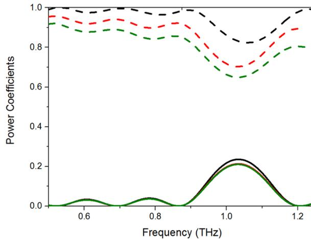
**Fig. 6.** Simulation results for ZnO-coated THz MMs with a coating thickness of 500 nm, as in the experiment (Fig. 3). Reflection (solid) and transmission (dashed) power coefficients for 7.29 (black),  $7.29 + 0.5i$  (red), and  $7.29 + 1.0i$  (green) ZnO permittivity.
