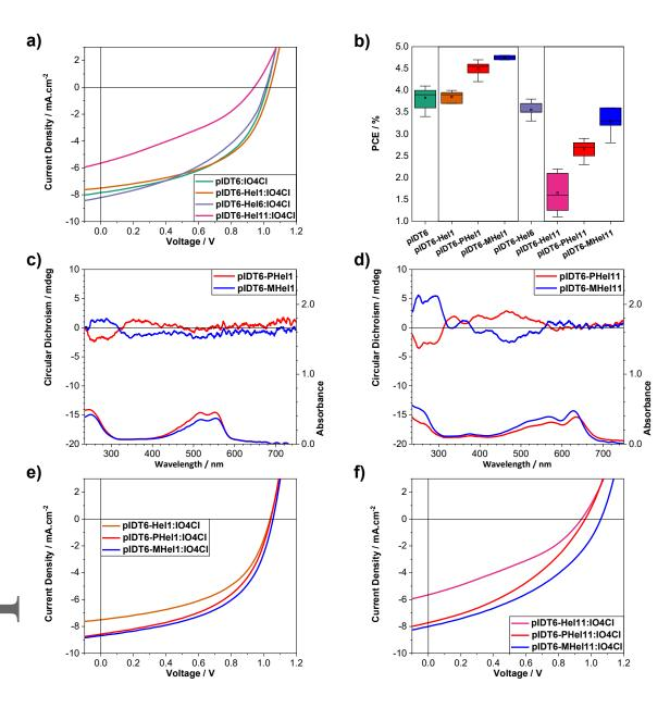
**Figure 4.** (a) *J-V* curves of the cells based on racemic polymers, (b) box plot of the PCE of all the solar cells studied. (c, d) ECD (top) and UV-Vis absorption spectra (bottom) of the thin-films blends of **pIDT6-(P/M)Hel1:IO4Cl** (c) and **pIDT6-(P/M)Hel1:IO4Cl** (d). (e, f) *J-V* curves of the cells based on racemic and enantiopure polymers on 1% helicene loading (e) and on 11% helicene loading (f).
