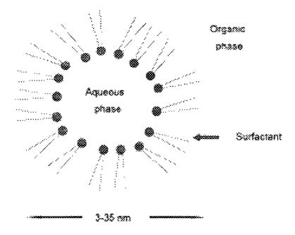
Fig. 1. Schematic presentation of reverse micelle.
