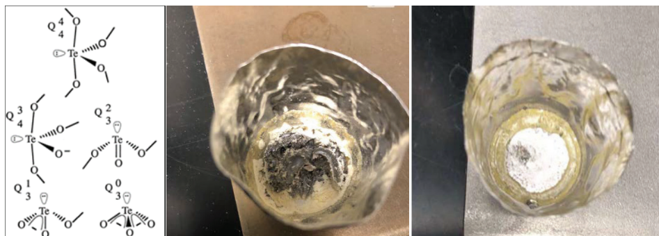
FIGURE 1. Left: Q_m^n , where m = 3,4 identifies the total number of oxygen bonded to the tellurium atom and n = 0-4 is the number of bridging oxygen bonded to the tellurium atom. 11 Right: Tellurium dioxide crystal (left). Pure tellurium dioxide glass made with IQ technique (right).
