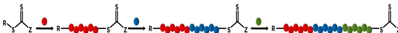
Scheme 1. Schematic representation of the synthesis of ABC-type triblock terpolymers via sequential RAFT polymerization. The red, blue and green dots stand for the three different monomers.
