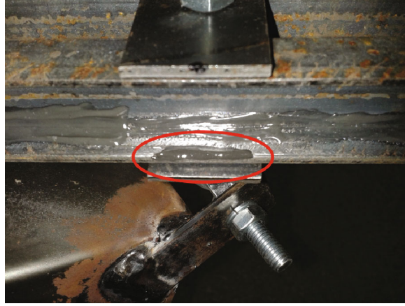
FIGURE 5: An FBG (circled) attached between the continuous Phase-OTDR fiber (top) and a corner reflector (bottom).
