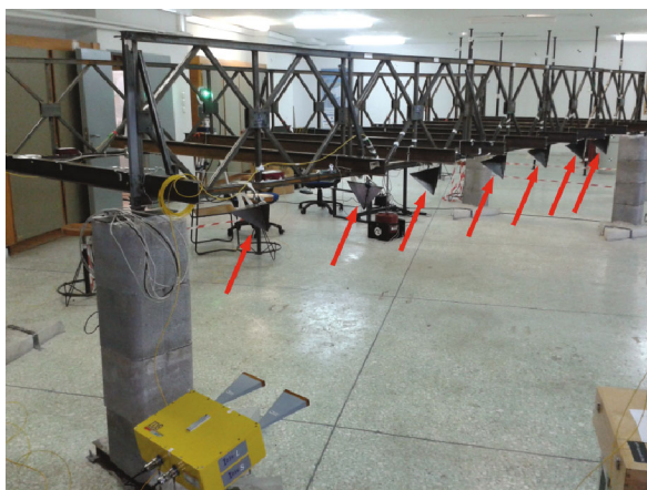
FIGURE 4: Picture of the installed GBRI system and the 7 CRs in the laboratory (indicated by the arrows).
