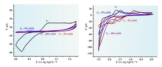
**Figure 5.** Cyclic voltammograms of the C2 systems for both the oxidation and the reduction process. in 0.1 mol  $L^{-1}$  Bu<sub>4</sub>NBF<sub>4</sub>. Scan rate 0.050 V s<sup>-1</sup>. Signals presented as: (red line) C3-3% rGO, (blue line) C3-5% rGO, and (purple line) C3-10% rGO.
