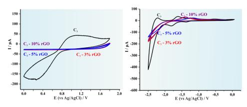
**Figure 6.** Cyclic voltammograms of the C3 systems for both the oxidation and the reduction process. in 0.1 mol  $L^{-1}$  Bu<sub>4</sub>NBF<sub>4</sub>. Scan rate 0.050 V s<sup>-1</sup>.
