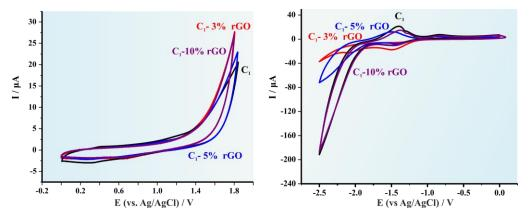
**Figure 4.** Cyclic voltammograms of the C1 systems for both the oxidation and the reduction process. in 0.1 mol  $L^{-1}$  Bu<sub>4</sub>NBF<sub>4</sub>. Scan rate 0.050 V s<sup>-1</sup>. Signals presented as: (red line) C1-3% rGO, (blue line) C1-5% rGO, and (purple line) C1-10% rGO.
