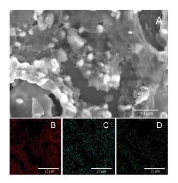
**Figure 2.** SEM images of a hybrid system with the Copolymer 2 and the rGO (**A**). There is an apparent intercalation that is supported with the aid of EDS, where the elemental mapping analysis confirms the existence of Carbon (**B**), Sulfur (**C**) and Oxygen (**D**).
