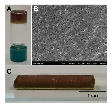
**Figure 4.** Fmoc-FF hydrogel encapsulating the Zn-T(MePy)P(I<sub>4</sub>) metalloporphyrin. (**A**) The hydrogel in a glass vial placed upside down; (**B**) fibrillar formation as observed by FESEM (scale-bar: 100 nm); (**C**) Fmoc-FF-[Zn-T(MePy)P(I<sub>4</sub>)] hydrogel shape integrity after being extruded from a syringe.
