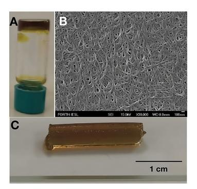
**Figure 3.** Fmoc-FF hydrogel encapsulating the Zn-T(MePy)P(Cl<sub>4</sub>) metalloporphyrin. (**A**) The hydrogel in a glass vial placed upside down; (**B**) fibrillar formation as observed by FESEM (scale bar: 100 nm); (**C**) Fmoc-FF-[Zn-T(MePy)P(Cl<sub>4</sub>)] hydrogel shape integrity after being extruded from a syringe.
