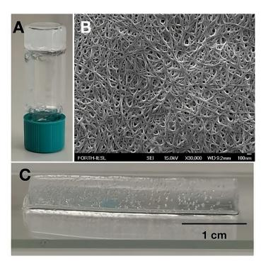
**Figure 1.** Fmoc-FF hydrogel. (**A**) The hydrogel in a glass vial placed upside down; (**B**) fibrillar formation as observed by FESEM (scale bar: 100 nm); (**C**) Fmoc-FF hydrogel shape integrity after being extruded from a syringe.
