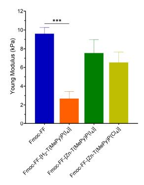
**Figure 5.** Determination of Young's modulus of the different hydrogels. Statistical analysis was performed compared to the control hydrogel Fmoc-FF using one-way ANOVA (\*\*\* p < 0.001).
