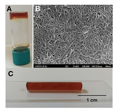
**Figure 2.** Fmoc-FF hydrogel encapsulating the H<sub>2</sub>-T(MePy)P(I<sub>4</sub>) porphyrin. (**A**) The hydrogel in a glass vial placed upside down; (**B**) fibrillar formation as observed by FESEM (scale bar: 100 nm); (**C**) Fmoc-FF-[H<sub>2</sub>-T(MePy)P(I<sub>4</sub>)], hydrogel shape integrity after being extruded from a syringe.
