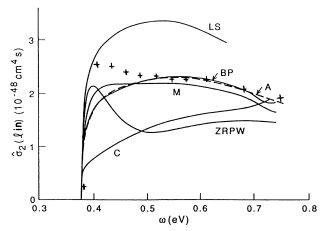
FIG. 1. Two-photon detachment cross sections as a function of laser field frequency  $\omega$ . This figure is taken from Fig. 4 of Geltman [14] with our results added (crosses). The initials are those used by Geltman [14]. They correspond to (C), Ref. [21]; (A), Ref. [7]; (LS), Ref. [24]; (best phase BP, model M, zerorange plane-wave ZRPW), Ref. [14].
